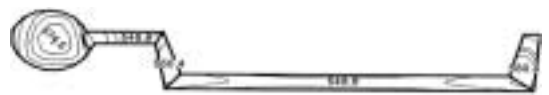
Fig. 6 Part temperature field at the end of solidification (14,8 seconds of cooling) considering Newtonian heat transfer at interface part/mould
